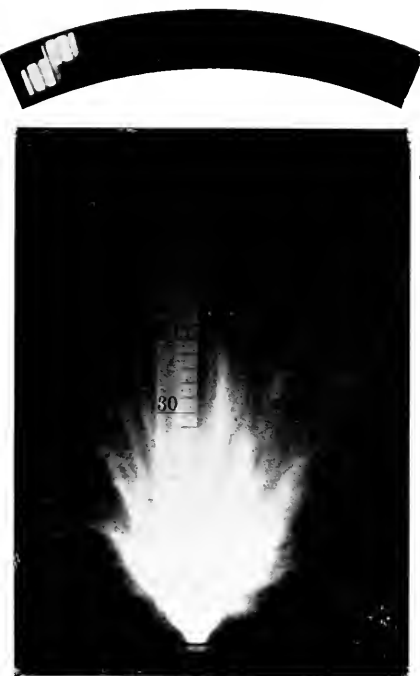
FIG. 136. Flame from Picric Acid with 5 per cent. Sodium Bicarbonate
